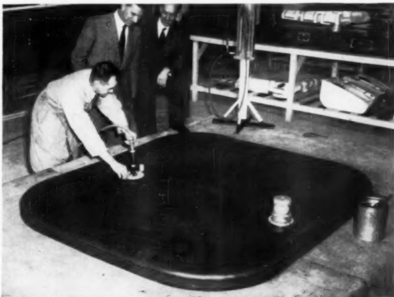
VENTING SYSTEM on 200 Imp. gal. synthetic rubber bag is about to be tested at plant of Dunlop Rubber Co., Melbourne. Bag withstands 100F at 20,000 ft.
